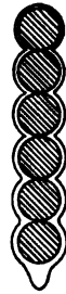
FIG. 33. — Diagram showing the adjustment of the capillary film in a long column and the appearance of free or gravitational water if the weight is too great for the supporting films.
